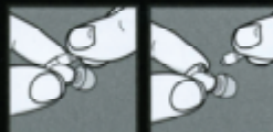
HOLD the earguns and cable firmly with each hand REMOVE the cable by holding close to the connection and pulling at a straight angle from the socket. Do not pull from the wires!
