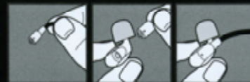
CHECK if the cable is for the left or right monitor MATCH the cable to the appropriate monitor INSERT the cable into the monitor by pushing it firmly into the socket
