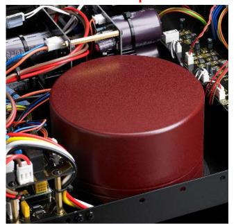
PDF Compressor Free Version The heart of the HINT 6's power supply is a massive 1.1 kVA toroid power transformer. It is custom designed for well-contained radiated hum, high efficiency, and high power. Encapsulating this massive power transformer in an epoxy-filled steel canister assures ultra-quiet performance.
