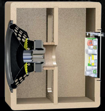
The extremely rigid, non-resonant cabinet of 1" MDF incorporates internal bracing of 3/4" MDF to reinforce the enclosure and support the powerful bass driver.
